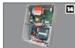
DC Converter Provides battery backup to the system
