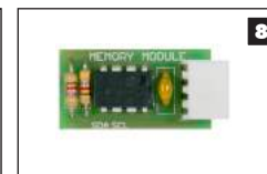
8 Backup memory module Back up all the transmitters and operating details set up in the controller
