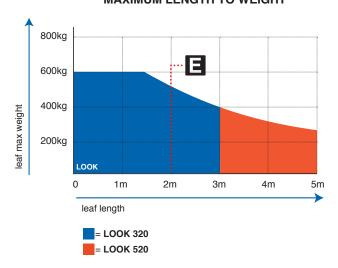
If gate leaf is greater than 2m, installing an electric-lock to the gate is strongly recommended.
